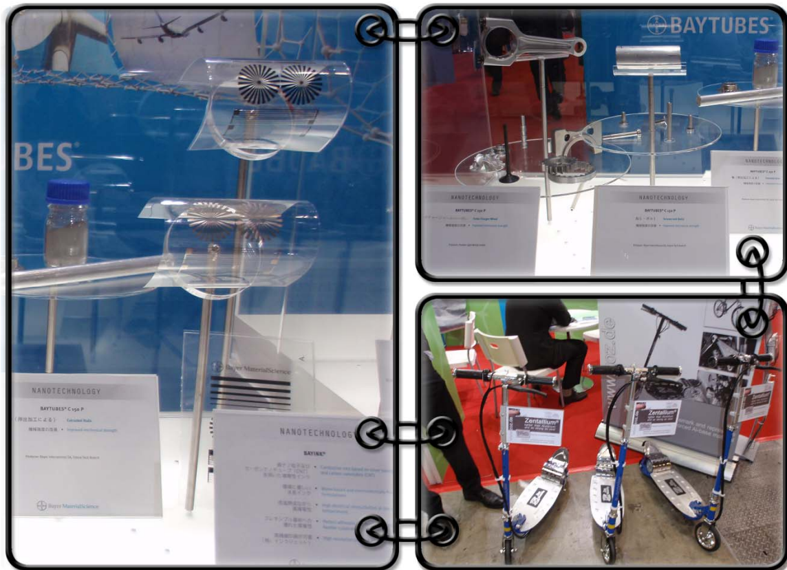
Fig. 1. Left: BayInk sample and the printed flexible conductive circuits on the transparent substrate; Top right: semi-finished products (rods and complex bars) as well as fasteners (nuts and bolts) made by Bayer CNT-Al composites, which is as strong as steel and as light as Aluminum; Bottom right: Zoz mobility vehicles using Zentallium.
