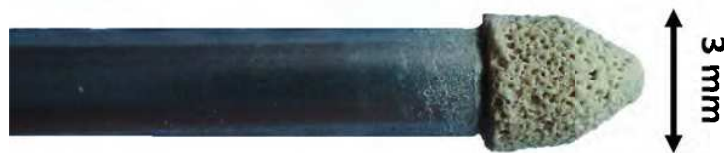
Figure 9. Polishing pen with head made of diamond-coated PUR foam; monocrystalline diamonds, grain size 8\text{-}12 \mu\text{m} .
