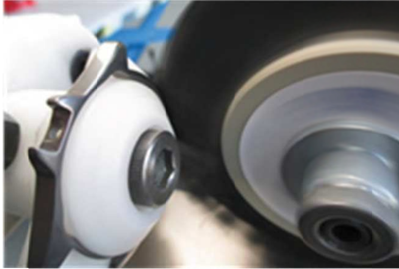
Figure 7. Soft brush finishing of a watch case (grey subject left hand); rotating brush (right hand).
