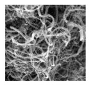
By adding agglomerations of carbon nanotubes to aluminium using powder metallurgy, it is possible to achieve tensile strength levels that almost match those of steel.
